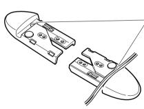
The slot for passing through the cable
